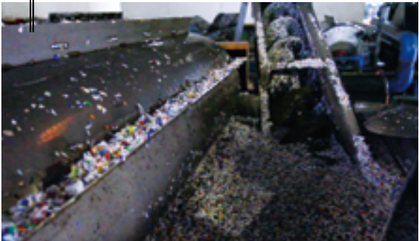
步驟一 Step 1 回收並分類膠樽，將其預洗及消毒後打成碎片。 Recycled bottles are first sorted, then washed, sterilized, and shredded into flakes.
